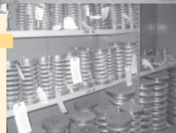
Spring assemblies to cover all set pressure ranges are offered.
